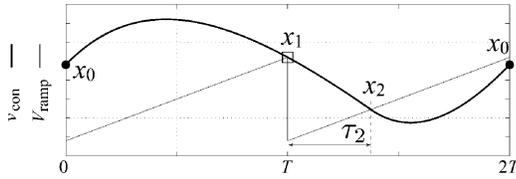
Fig. 5. Border collision (Bc2a) of period-2 solution.
