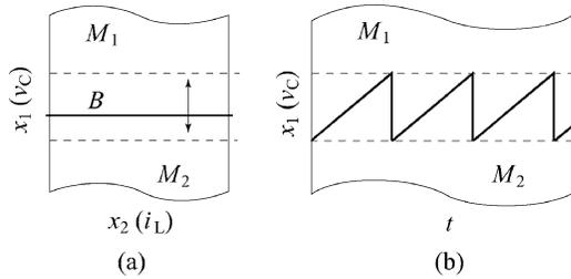
Fig. 2. Periodically moving border in the buck converter.
