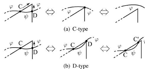
Fig. 4. Classification of border collision in buck converter.
